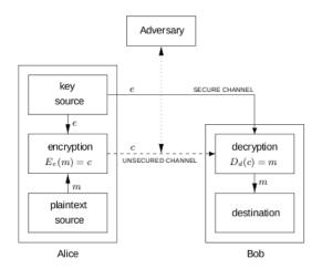
**Figure 1.7:** Two-party communication using encryption, with a secure channel for key exchange. The decryption key d can be efficiently computed from the encryption key e.
