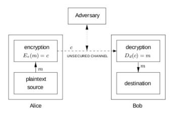
Figure 1.6: Schematic of a two-party communication using encryption.
