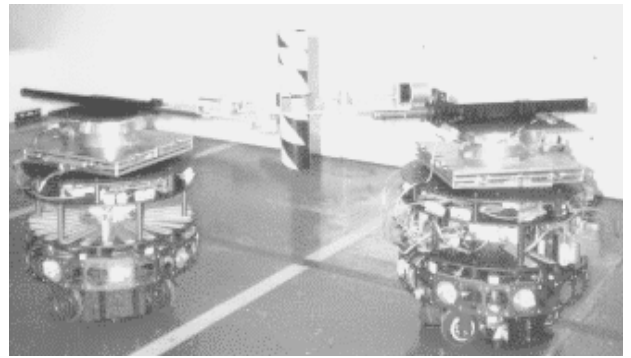
Figure 6: Fred and Ginger with capture-heads, manipulators, ultra-sonic and beacon sensors.
