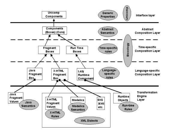
Figure 6. The layered architecture of COMPOST.
