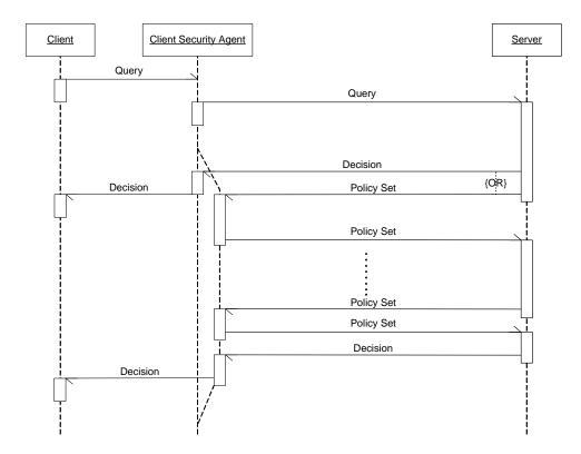
Figure 2: Sequence Diagram for an Access Control Query
