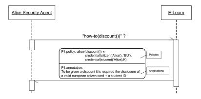
Figure 7: Example Sequence Diagram of a How-To Query
