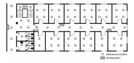
Figure 10: Radio map with several access points and reference points [3]
