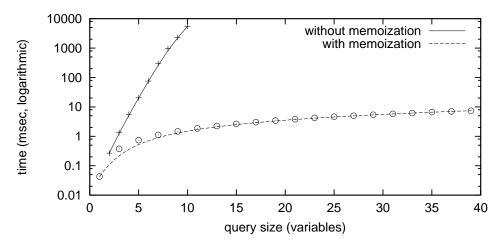
Figure 1: Effect of Memoization over Query Size (data synthetic, uniform, deeply nested; bindings for query variables overlap considerably)
