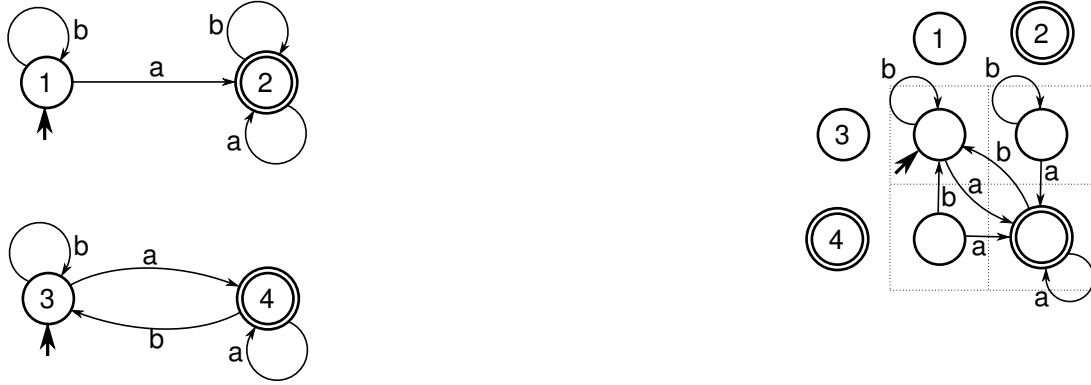
Figure 6.2: The product automaton on the right accepts the intersection of the language of the two automata on the left.
