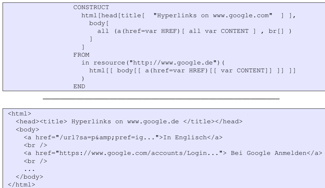
Figure 2.8: Above the line an Xcerpt rule is given. It is conceived to retrieve all the hyperlinks from the start page of Google and to present them in a plain HTML document. The result of evaluating the rule is shown below the line—this time not in Xcerpt data term syntax, but in XML (and hence XHTML) syntax.
