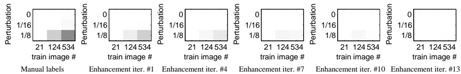
Figure 7: The convergence rate of fitting using an AAM trained from manual labels, and AAM after enhancement iteration number 1, 4, 7, 10 and 13. Continuing improvement of fitting performance is observed as the enhancement process progresses.
