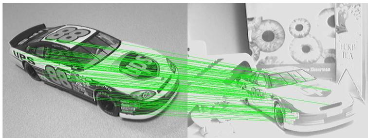
Figure 5: *Feature matching under extreme illumination conditions.* About 40% of the 200 selected features are well matched despite strong saturation and reflection.
