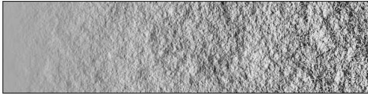
Fig. 4. Sayles surface: the effect of varying surface roughness.
