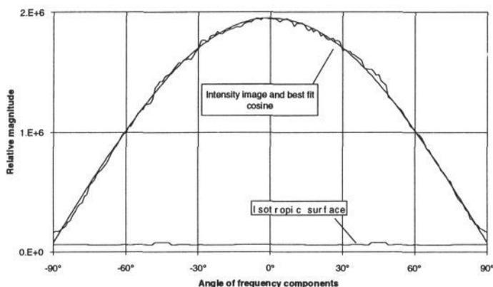
Figure 3- Polar frequency plot of image texture ( $\tau = 0^\circ$ ), and corresponding best fit cosine (original surface also shown).
