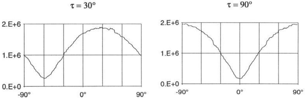
Figure 5 - Polar frequency plots of image texture showing the effect of variation in illuminant tilt ( $\tau$ ). Axes are as figure 3.
