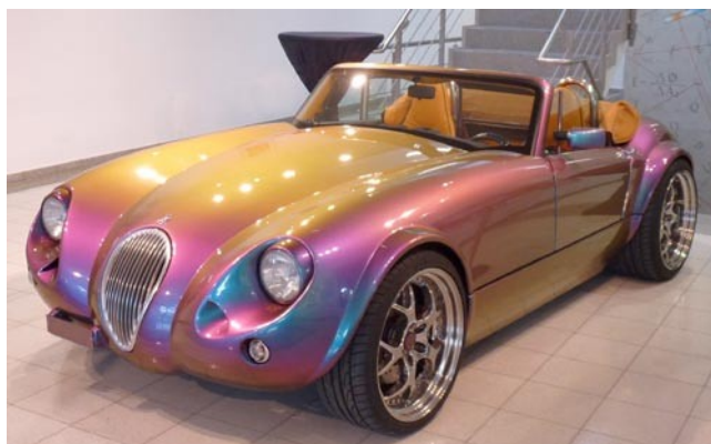
Figure 1. Car painted with special-effect varnishing "Metallic Fantasy Emerald Green", according to the visual perspective and the light conditions, the colour impression changes.
