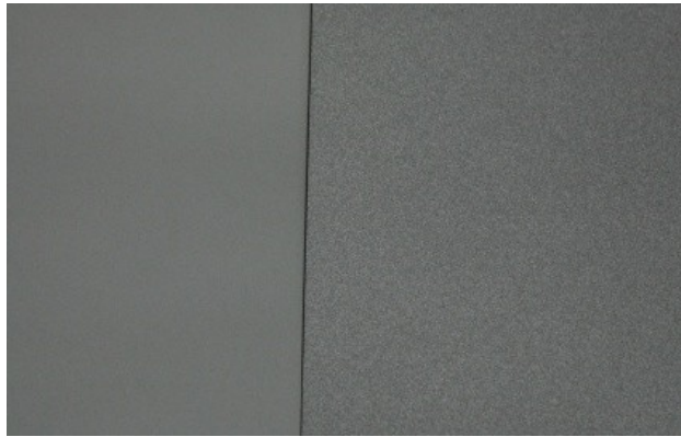
Figure 1. Two car paint samples under diffuse lighting conditions. The samples differ in the texture parameter Diffuse Coarseness
