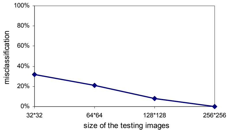
Figure 7. 10 Misclassification rate for 4 synthetic textures against the size of the test samples.
