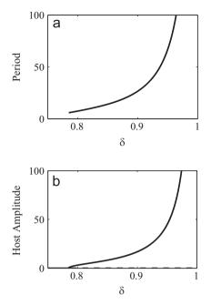
**Fig. 1.** In (a) the period of the limit cycles is plotted as  $\delta$  is varied. In (b) the amplitudes of the steady state and the limit cycles are plotted as  $\delta$  is varied. Stability and instability are indicated by the solid and dashed lines respectively. All other parameter values are kept constant with the following values: a=1.7,  $\beta = \gamma = 10/1.05$ ,  $\mu = 1.0003/1.05$  and k=1.
