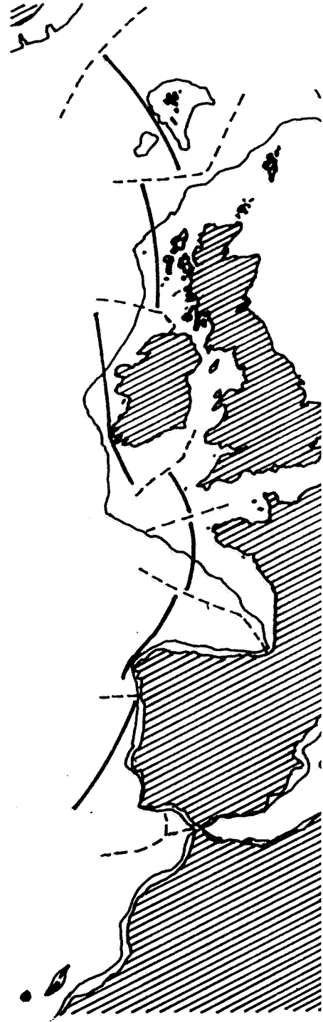
Figure 7.3 Tentative lines for the maximum exploitation of Europe's Atlantic wave power resource with international sea bed boundaries (---).
