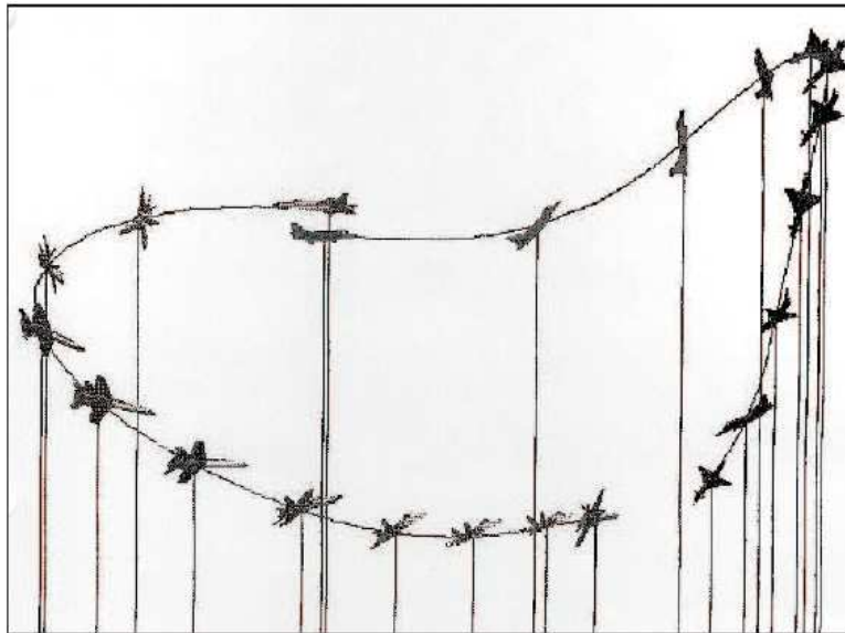
Figure 2. A example of a novel maneuver evolved by the learning classifier system under the HSHP starting condition (see figure 1). The aircraft on the left is following a fixed, but reactive strategy; the aircraft on the right is following a strategy evolved by the LCS, which in turn is a new variation on the Herbst maneuver.
