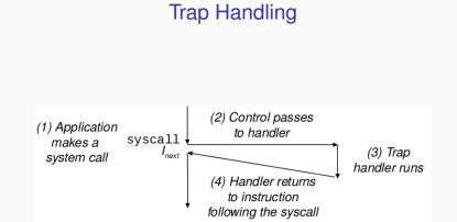
The trap handler returns control to the next instruction in the application program's control flow.
