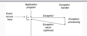
A change in the processor's state (event) triggers an abrupt control transfer (an **exception**) from the application program to an exception handler. After it finishes processing, the handler either returns control to the interrupted program or aborts.
