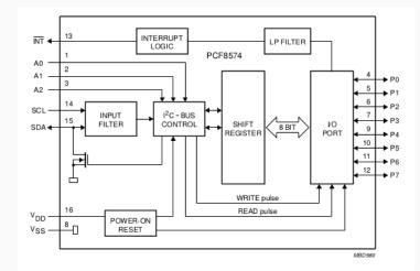
NB: 1 input data channel (SDA), 8 output data channels (P0 ... P7)
