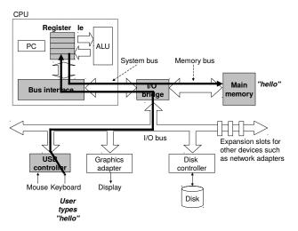
The shell reads ./hello from the keyboard, stores it in memory; then, initiates to load the executable file from disk to memory. <sup>0</sup>From Bryant and O'Hallaron, Ch 1
