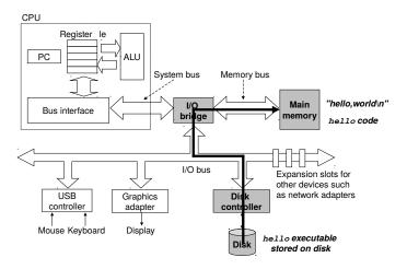
Using direct memory access (DMA) the data travels from disk directly to memory.
