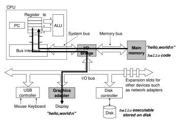
Once the code and data in the hello object file are loaded into memory, the processor begins executing the machine-language instructions in the hello program's main routine.
