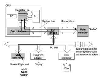
The shell reads ./hello from the keyboard, stores it in memory; then, initiates to load the executable file from disk to memory.
