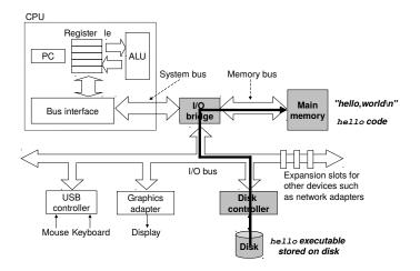
Using direct memory access (DMA) the data travels from disk directly room to memory.
