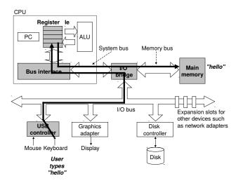
The shell reads ./hello from the keyboard, stores it in memory; then, initiates to load the executable file from disk to memory.
