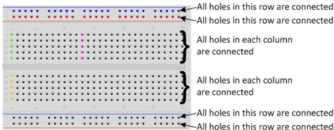
Using a breadboard, like the one above, simplifies the wiring, especially for larger projects (as in CW2).
