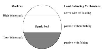
Fig. 16. Low- and high-watermark mechanisms for spark distribution. (showing a single spark pool). By default work-stealing (passive) load distribution is used. If the size exceeds the higher-watermark, work is actively offloaded. The system aims to always fill the pool up to the low-watermark.
