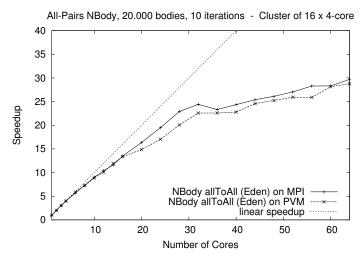
Fig. 18. NBody (Eden): 20000 particles, 10 iterations
