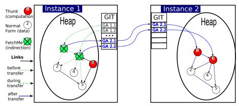
Fig. 11. Transferring graph structures between PAEAN instances. Here, the sub-graph rooted at address 1 (with GA2.1) has been transferred from instance 1 to instance 2. Thunks are moved, replacing them by *FetchMes* on instance 1, while normal forms are copied. GA1.1 and GA1.2 are only used during transfer. At completion of the transfer, they are replaced by GA2.1 and GA2.2.
