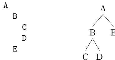
Figure 4.3: An example of Kofler's printing function output (left), and the parse tree it represents (right)
