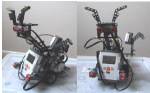
Fig. 3. Lego robot, expressing artificial emotions using a combination of two basic movements of its body: moving the 'neck' forward/backward, and raising/lowering 'eyebrows'.
