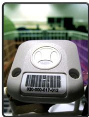
Figure 1. A Ubisense tag. Players used the tag button to record game events.
