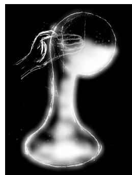
Figure 1. Intelligent lamp sketch. Light in this lamp is 'fluid' and can proactively follow an object, such as a book. It can also 'stick' to the hand, and that way be manually directed and distributed over the lamp. A design hypothesis was that the lamp invited Creativity related behaviours by offering an easy possibility to create lighting patterns on the lamp using the hand.
