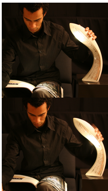
Figure 3. Side view of the fully functional intelligent lamp. A Power LED array enables light beams in multiple directions. It uses a miniature camera for object tracking and has a touch sensitive top surface for manipulation of the light. The lamp is connected to a Powerbook G4 running Max/MSP, which controls its behaviour and does the image processing.
