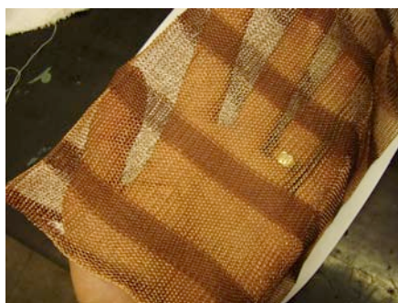
Figure 1. Example of Vertically Embedded Conductive Bands
