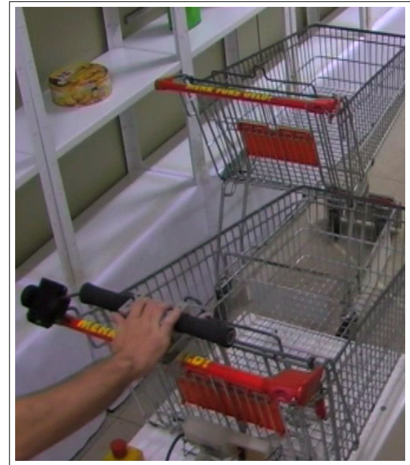
Figure 11. The user is steering InBOT like an ordinary shopping cart using the handle. Because he needs his left hand otherwise he grabs the handle with his right hand only. This makes it difficult for him to maneuver dexterously. So the user benefits from being supported by the obstacle avoidance of the basic behavior repertoire .
