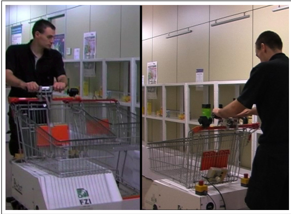
Figure 10. The user is steering InBOT like an ordinary shopping cart using the handle. He is supported by InBOT's motors.
