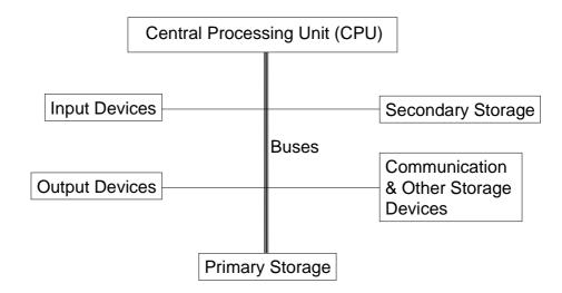
The CPU has a von Neumann architecture and consists of a Control Unit, an Arithmetic and Logic Unit (ALU) and various Registers. The Control Unit can load values into the Registers for processing by the ALU and also use the values stored in the Registers to address memory locations.
