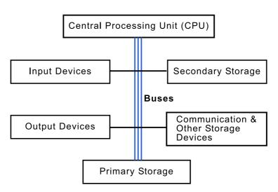
The CPU has a von Neumann architecture and consists of a Control Unit, an Arithmetic and Logic Unit (ALU) and various Registers. The Control Unit can load values into the Registers for processing by the ALU and also use the values stored in the Registers to address memory locations.
