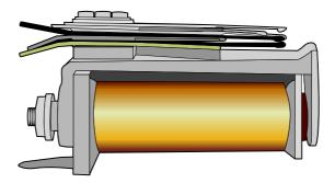
Konrad Zuse's Z1-Z4 machines (1934-45) and the Harvard Mark I (due to Howard Aiken in 1944) used electro-magnetic relays as their switches. This continued dependence on mechanical components meant that the machines remained large and unreliable (as well as rather noisy!).
