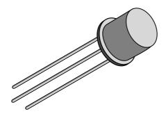
In 1947 Bardeen, Brattain and Shockley of Bell Labs invented the transistor. This device which was smaller, cheaper, faster and more reliable than the valve ushered in the second generation of computers.
