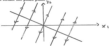
Clearly  $\frac{dx}{dt} > 0$  whenever x > -2y and so the trajectories are in the direction shown.
