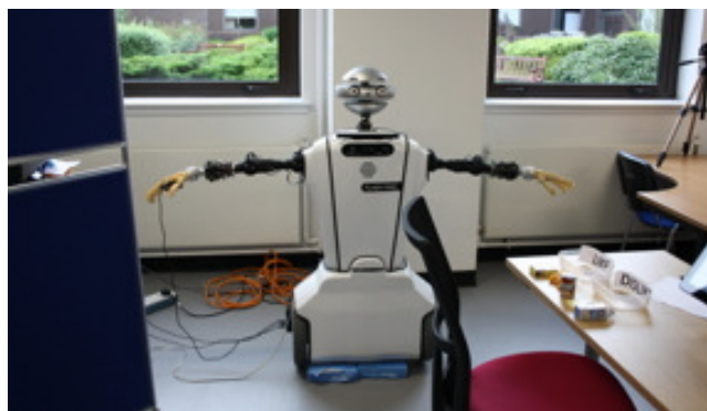
Figure 4: Emotion recognition task setup. RFID reader strapped to robots right hand. RFID tagged items on table.
