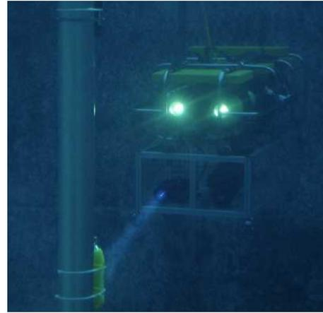
Figure 2: Typical ROV inspection operation of a riser with a fluorometer sensor.
