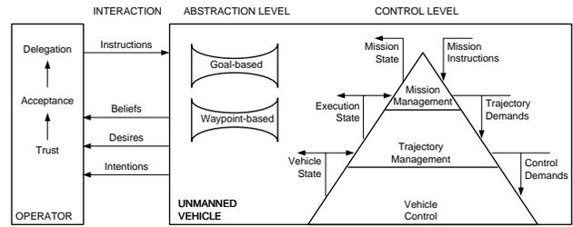
Figure 5: Levels of control related to the level of abstraction of knowledge for operator's delegation of tasks to unmanned vehicles.
