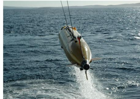
Figure 3: AUV recovery after finishing a mission (courtesy of SeeByte Ltd.).
