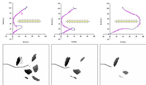
Figure 8: Top: Net avoidance trajectories obtained with the dynamic model simulator. Bottom : Three sequential observations of the local map with trail showing planned forward trajectory to achieve the waypoint in a real scenario.
