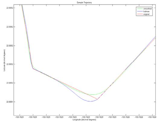
Figure 7: Original, Kalman filtered and RTS smoothed trajectory of an underwater vehicle.
