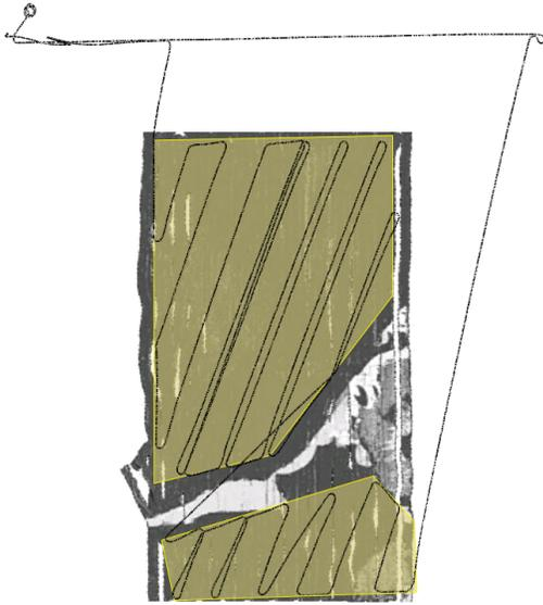
Figure 9: AUV survey of two seabed areas with an adaptive mission planner capable of reacting to water currents and sensor faults.
