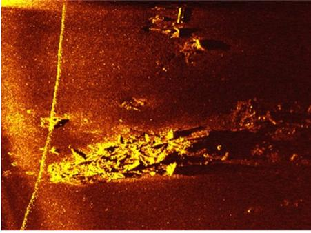
Figure 1: Acoustic image of 50m range of a WWI U-boat sunk in Hoxa Sound, Scapa Flow (courtesy of SeeByte Ltd.).
