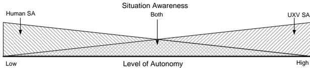
Figure 4: Human and AUV SA across the levels of autonomy
