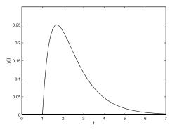
FIGURE 4.1. The mass sits in the equilibrium position y = 0 until it is hit by the hammer at  $t = t_0$  (as an example we took  $t_0 = 1$  above). Note that the values for the mass, coefficient of friction and spring stiffness mean that we are in the overdamped case.
