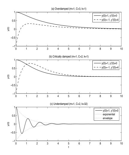
FIGURE 2.1. Overdamping, critical damping and underdamping for a simple mass-spring system. We used the specific values for m, C and k shown. In (a) and (b) we plotted the two solutions corresponding to the two distinct sets of initial conditions shown.
