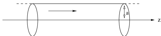
Fig. 19 Poiseuille flow: a viscous fluid flows along an infinite horizontal pipe with circular cross-section of radius a , whose centre line is aligned along the z -axis. A constant pressure gradient is assumed, as well as axisymmetry, no radial flow and no swirl.
